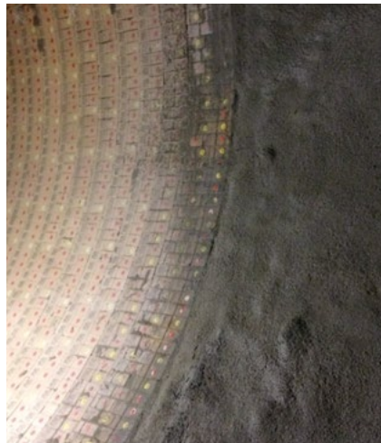
Figure 1/2: Insights into practice: Veneering of a hot spot (Fig. 1) and a protective layer in full circumference (Fig. 2), both kilns with a diameter > 5.00 m.
